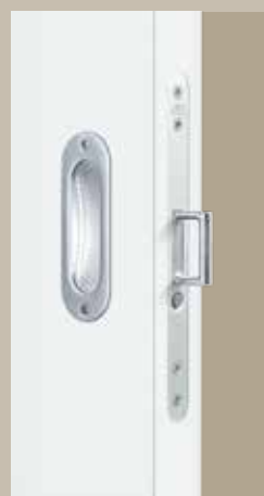
For sliding doors that run within the wall, you can conceal the door leaf completely in the wall with a trip handle. The handle springs out at the press of a button, allowing you to close the door.
