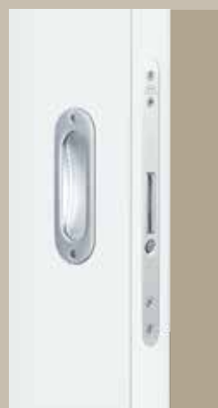
For sliding doors that run within the wall, you can conceal the door leaf completely in the wall with a trip handle. The handle springs out at the press of a button, allowing you to close the door.
